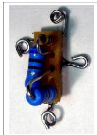
Picture 16 The Bi Color Signal is mounted near the turnout. The 4 terminal resistor assembly is connected below the two wire Turnout signal. Note that the two 680 Ohm 1.2 W are larger and the one 360 Ohm 1/4 W is smaller. The Blue wire and Flag wire both connect the terminal on the left, White wire on the right, and positive on the bottom. (digikey.com PPC680LCT-ND 680 Ohms 1/2 W, and P360CACT-ND 360 Ohms 1/4 W)
