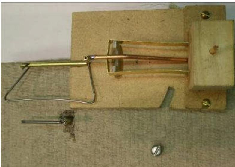
Picture 2 The "U" Toggle assembly is easy to take out and put back into place. Note that when the wire is in the center, both electrical contacts are not closed.
